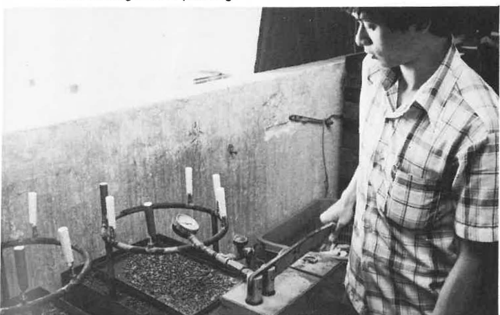
"Elite" brand disposable cigarette lighter, a product of Chiap Hua Clocks & Watches Ltd., has recently been awarded the HKQ-mark. Picture shows a hydrostatic test being done on the lighter before assembly.
